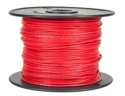
Atlas Wire AWM hook-up wire, single conductor, 22 AWG, 7-stranded, tinned copper, PVC conductor insulation material, red, 300V, 1000ft spool.
