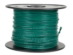
Atlas Wire AWM hook-up wire, single conductor, 22 AWG, 7-stranded, tinned copper, PVC conductor insulation material, green, 300V, 1000ft spool.
