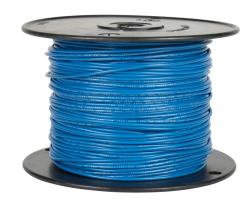
Atlas Wire AWM hook-up wire, single conductor, 22 AWG, 7-stranded, tinned copper, PVC conductor insulation material, blue, 300V, 1000ft spool.
