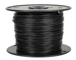
Atlas Wire AWM hook-up wire, single conductor, 22 AWG, 7-stranded, tinned copper, PVC conductor insulation material, black, 300V, 1000ft spool.
