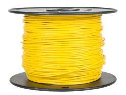
Atlas Wire AWM hook-up wire, single conductor, 20 AWG, 10-stranded, tinned copper, PVC conductor insulation material, yellow, 300V, 500ft spool.
