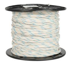
Atlas Wire AWM hook-up wire, single conductor, 20 AWG, 10-stranded, tinned copper, PVC conductor insulation material, white with blue stripe, 300V, 500ft spool.
