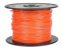
Atlas Wire AWM hook-up wire, single conductor, 20 AWG, 10-stranded, tinned copper, PVC conductor insulation material, orange, 300V, 500ft spool.
