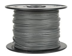
Atlas Wire AWM hook-up wire, single conductor, 20 AWG, 10-stranded, tinned copper, PVC conductor insulation material, gray, 300V, 500ft spool.
