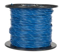
Atlas Wire AWM hook-up wire, single conductor, 20 AWG, 10-stranded, tinned copper, PVC conductor insulation material, blue with white stripe, 300V, 500ft spool.
