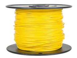
Atlas Wire AWM hook-up wire, single conductor, 18 AWG, 16-stranded, tinned copper, PVC conductor insulation material, yellow, 300V, 500ft spool.
