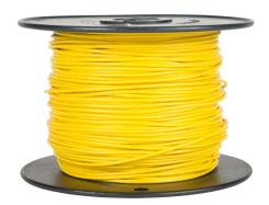
Atlas Wire AWM hook-up wire, single conductor, 18 AWG, 16-stranded, tinned copper, PVC conductor insulation material, yellow, 300V, 500ft spool.
