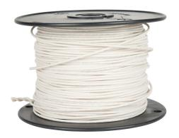
Atlas Wire AWM hook-up wire, single conductor, 18 AWG, 16-stranded, tinned copper, PVC conductor insulation material, white, 300V, 500ft spool.
