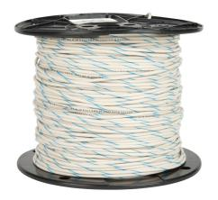
Atlas Wire AWM hook-up wire, single conductor, 18 AWG, 16-stranded, tinned copper, PVC conductor insulation material, white with blue stripe, 300V, 500ft spool.
