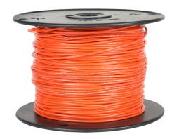
Atlas Wire AWM hook-up wire, single conductor, 18 AWG, 16-stranded, tinned copper, PVC conductor insulation material, orange, 300V, 500ft spool.
