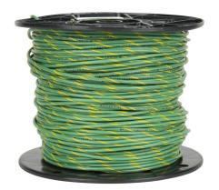
Atlas Wire AWM hook-up wire, single conductor, 18 AWG, 16-stranded, tinned copper, PVC conductor insulation material, green with yellow stripe, 300V, 500ft spool.
