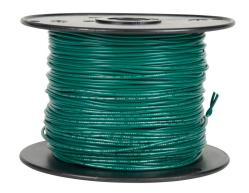
Atlas Wire AWM hook-up wire, single conductor, 18 AWG, 16-stranded, tinned copper, PVC conductor insulation material, green, 300V, 500ft spool.
