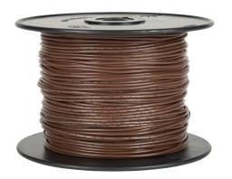
Atlas Wire AWM hook-up wire, single conductor, 18 AWG, 16-stranded, tinned copper, PVC conductor insulation material, brown, 300V, 500ft spool.
