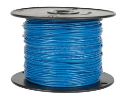
Atlas Wire AWM hook-up wire, single conductor, 18 AWG, 16-stranded, tinned copper, PVC conductor insulation material, blue, 300V, 500ft spool.
