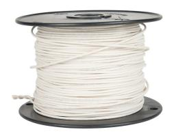
Atlas Wire AWM hook-up wire, single conductor, 16 AWG, 26-stranded, tinned copper, PVC conductor insulation material, white, 300V, 500ft spool.
