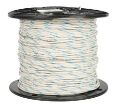
Atlas Wire AWM hook-up wire, single conductor, 16 AWG, 26-stranded, tinned copper, PVC conductor insulation material, white with blue stripe, 300V, 500ft spool.
