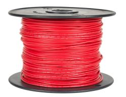
Atlas Wire AWM hook-up wire, single conductor, 16 AWG, 26-stranded, tinned copper, PVC conductor insulation material, red, 300V, 500ft spool.
