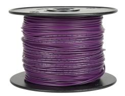
Atlas Wire AWM hook-up wire, single conductor, 16 AWG, 26-stranded, tinned copper, PVC conductor insulation material, purple, 300V, 500ft spool.
