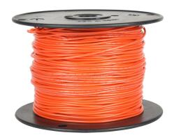
Atlas Wire AWM hook-up wire, single conductor, 16 AWG, 26-stranded, tinned copper, PVC conductor insulation material, orange, 300V, 500ft spool.
