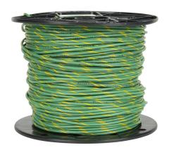
Atlas Wire AWM hook-up wire, single conductor, 16 AWG, 26-stranded, tinned copper, PVC conductor insulation material, green with yellow stripe, 300V, 500ft spool.
