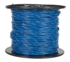
Atlas Wire AWM hook-up wire, single conductor, 16 AWG, 26-stranded, tinned copper, PVC conductor insulation material, blue with white stripe, 300V, 500ft spool.
