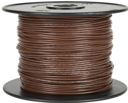
Atlas Wire AWM hook-up wire, single conductor, 16 AWG, 26-stranded, tinned copper, PVC conductor insulation material, brown, 300V, 500ft spool.
