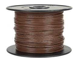
Atlas Wire AWM hook-up wire, single conductor, 16 AWG, 26-stranded, tinned copper, PVC conductor insulation material, brown, 300V, 500ft spool.
