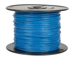
Atlas Wire AWM hook-up wire, single conductor, 16 AWG, 26-stranded, tinned copper, PVC conductor insulation material, blue, 300V, 500ft spool.
