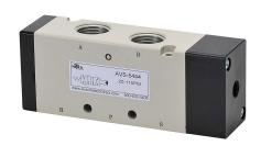
NITRA pilot valve, 5-port (4-way), 2-position, single air pilot spring return, (1) 1/2in female NPT inlet(s), (2) 1/2in female NPT outlet(s), (2) 1/2in female NPT exhaust(s), Cv=2.79.
