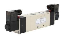
NITRA solenoid valve, 5-port (4-way), 3-position, center exhaust, double solenoid, (1) 1/2in female NPT inlet(s), (2) 1/2in female NPT outlet(s), (2) 1/2in female NPT exhaust(s), Cv=1.68, 24 VDC, 3.0W, 11mm DIN style wiring plug.
