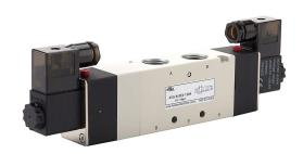
NITRA solenoid valve, 5-port (4-way), 3-position, center exhaust, double solenoid, (1) 1/2in female NPT inlet(s), (2) 1/2in female NPT outlet(s), (2) 1/2in female NPT exhaust(s), Cv=1.68, 120 VAC, 4.5VA, 11mm DIN style wiring plug.
