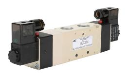
NITRA solenoid valve, 5-port (4-way), 3-position, center closed, double solenoid, (1) 1/2in female NPT inlet(s), (2) 1/2in female NPT outlet(s), (2) 1/2in female NPT exhaust(s), Cv=1.68, 24 VDC, 3.0W, 11mm DIN style wiring plug.
