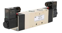
NITRA solenoid valve, 5-port (4-way), 3-position, center closed, double solenoid, (1) 1/2in female NPT inlet(s), (2) 1/2in female NPT outlet(s), (2) 1/2in female NPT exhaust(s), Cv=1.68, 24 VDC, 3.0W, 11mm DIN style wiring plug.
