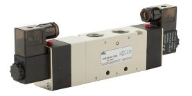
NITRA solenoid valve, 5-port (4-way), 3-position, center closed, double solenoid, (1) 1/2in female NPT inlet(s), (2) 1/2in female NPT outlet(s), (2) 1/2in female NPT exhaust(s), Cv=1.68, 120 VAC, 4.5VA, 11mm DIN style wiring plug.
