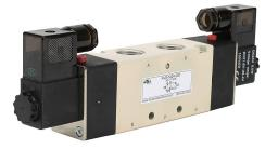
NITRA solenoid valve, 5-port (4-way), 2-position, double solenoid, (1) 1/2in female NPT inlet(s), (2) 1/2in female NPT outlet(s), (2) 1/2in female NPT exhaust(s), Cv=2.79, 24 VDC, 3.0W, 11mm DIN style wiring plug.
