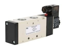
NITRA solenoid valve, 5-port (4-way), 2-position, single solenoid spring return, (1) 1/2in female NPT inlet(s), (2) 1/2in female NPT outlet(s), (2) 1/2in female NPT exhaust(s), Cv=2.79, 24 VDC, 3.0W, 11mm DIN style wiring plug.
