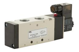
NITRA solenoid valve, 5-port (4-way), 2-position, single solenoid spring return, (1) 1/2in female NPT inlet(s), (2) 1/2in female NPT outlet(s), (2) 1/2in female NPT exhaust(s), Cv=2.79, 120 VAC, 4.5VA, 11mm DIN style wiring plug.
