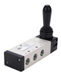
NITRA pneumatic manual valve, 5-port (4-way), 3-position, center exhaust, 90 deg hand lever, spring return, 1/4in female NPT inlet(s), 1/4in female NPT outlet(s), 1/4in female NPT exhaust(s), Cv=1, panel or surface mount.
