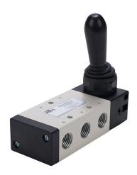
NITRA pneumatic manual valve, 5-port (4-way), 3-position, center exhaust, 90 deg hand lever, detented, 1/4in female NPT inlet(s), 1/4in female NPT outlet(s), 1/4in female NPT exhaust(s), Cv=1, panel or surface mount.
