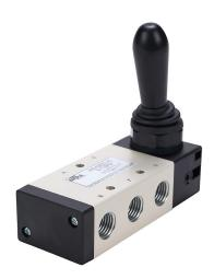
NITRA pneumatic manual valve, 5-port (4-way), 3-position, center closed, 90 deg hand lever, detented, 1/4in female NPT inlet(s), 1/4in female NPT outlet(s), 1/4in female NPT exhaust(s), Cv=1, panel or surface mount.
