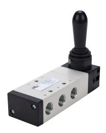
NITRA manual valve, 5-port (4-way), 3-position, center closed, handle, spring return, 1/4in female NPT inlet(s), 1/4in female NPT outlet(s), 1/4in female NPT exhaust(s), Cv=1, panel or surface mount.
