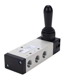
NITRA pneumatic manual valve, 5-port (4-way), 3-position, center closed, 90 deg hand lever, spring return, 1/4in female NPT inlet(s), 1/4in female NPT outlet(s), 1/4in female NPT exhaust(s), Cv=1, panel or surface mount.
