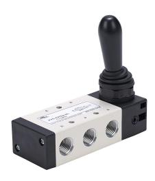
NITRA manual valve, 5-port (4-way), 2-position, handle, detented, 1/4in female NPT inlet(s), 1/4in female NPT outlet(s), Cv=1.39, panel or surface mount.
