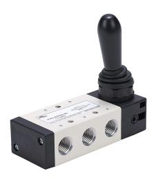
NITRA pneumatic manual valve, 5-port (4-way), 2-position, 90 deg hand lever, detented, 1/4in female NPT inlet(s), 1/4in female NPT outlet(s), Cv=1.39, panel or surface mount.
