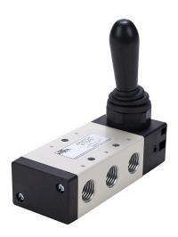
NITRA manual valve, 5-port (4-way), 2-position, handle, spring return, 1/4in female NPT inlet(s), 1/4in female NPT outlet(s), 1/4in female NPT exhaust(s), Cv=1.39, panel or surface mount.
