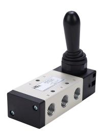
NITRA pneumatic manual valve, 5-port (4-way), 2-position, 90 deg hand lever, spring return, 1/4in female NPT inlet(s), 1/4in female NPT outlet(s), 1/4in female NPT exhaust(s), Cv=1.39, panel or surface mount.
