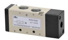
NITRA pilot valve, 5-port (4-way), 2-position, single air pilot spring return, (1) 3/8in female NPT inlet(s), (2) 3/8in female NPT outlet(s), (2) 1/4in female NPT exhaust(s), Cv=1.67.
