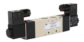
NITRA solenoid valve, 5-port (4-way), 3-position, center exhaust, double solenoid, (1) 3/8in female NPT inlet(s), (2) 3/8in female NPT outlet(s), (2) 1/4in female NPT exhaust(s), Cv=1, 24 VDC, 3.0W, 11mm DIN style wiring plug.
