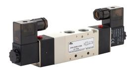
NITRA solenoid valve, 5-port (4-way), 3-position, center exhaust, double solenoid, (1) 3/8in female NPT inlet(s), (2) 3/8in female NPT outlet(s), (2) 1/4in female NPT exhaust(s), Cv=1, 120 VAC, 4.5VA, 11mm DIN style wiring plug.
