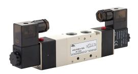
NITRA solenoid valve, 5-port (4-way), 3-position, center exhaust, double solenoid, (1) 3/8in female NPT inlet(s), (2) 3/8in female NPT outlet(s), (2) 1/4in female NPT exhaust(s), Cv=1, 120 VAC, 4.5VA, 11mm DIN style wiring plug.
