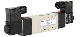
NITRA solenoid valve, 5-port (4-way), 3-position, center exhaust, double solenoid, (1) 1/4in female NPT inlet(s), (2) 1/4in female NPT outlet(s), (2) 1/4in female NPT exhaust(s), Cv=1, 24 VDC, 3.0W, 11mm DIN style wiring plug.
