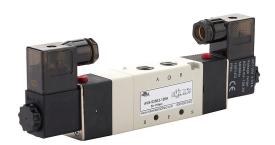
NITRA solenoid valve, 5-port (4-way), 3-position, center exhaust, double solenoid, (1) 1/4in female NPT inlet(s), (2) 1/4in female NPT outlet(s), (2) 1/4in female NPT exhaust(s), Cv=1, 120 VAC, 4.5VA, 11mm DIN style wiring plug.
