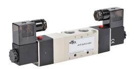
NITRA solenoid valve, 5-port (4-way), 3-position, center closed, double solenoid, (1) 3/8in female NPT inlet(s), (2) 3/8in female NPT outlet(s), (2) 1/4in female NPT exhaust(s), Cv=1, 24 VDC, 3.0W, 11mm DIN style wiring plug.
