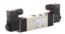
NITRA solenoid valve, 5-port (4-way), 3-position, center closed, double solenoid, (1) 3/8in female NPT inlet(s), (2) 3/8in female NPT outlet(s), (2) 1/4in female NPT exhaust(s), Cv=1, 120 VAC, 4.5VA, 11mm DIN style wiring plug.
