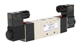
NITRA solenoid valve, 5-port (4-way), 3-position, center closed, double solenoid, (1) 1/4in female NPT inlet(s), (2) 1/4in female NPT outlet(s), (2) 1/4in female NPT exhaust(s), Cv=1, 24 VDC, 3.0W, 11mm DIN style wiring plug.
