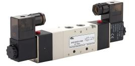
NITRA solenoid valve, 5-port (4-way), 3-position, center closed, double solenoid, (1) 1/4in female NPT inlet(s), (2) 1/4in female NPT outlet(s), (2) 1/4in female NPT exhaust(s), Cv=1, 120 VAC, 4.5VA, 11mm DIN style wiring plug.
