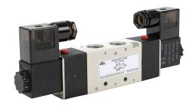
NITRA solenoid valve, 5-port (4-way), 2-position, double solenoid, (1) 3/8in female NPT inlet(s), (2) 3/8in female NPT outlet(s), (2) 1/4in female NPT exhaust(s), Cv=1.68, 24 VDC, 3.0W, 11mm DIN style wiring plug.
